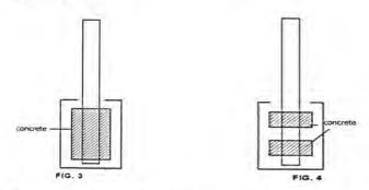
**9.2.2.3.3 Method 3.** Tap the post into the bottom of the hole until the desired height of the post above ground level is reached (see Fig. 4). Fill the hole one fourth of the depth with concrete, then add fine rocks or gravel to one half of the depth of the hole, then add concrete to three fourths of the depth of the hole. Fill the remainder of the hole with soil, gravel, or fine rocks. Check to see that the post remains plumb until the concrete has set.
