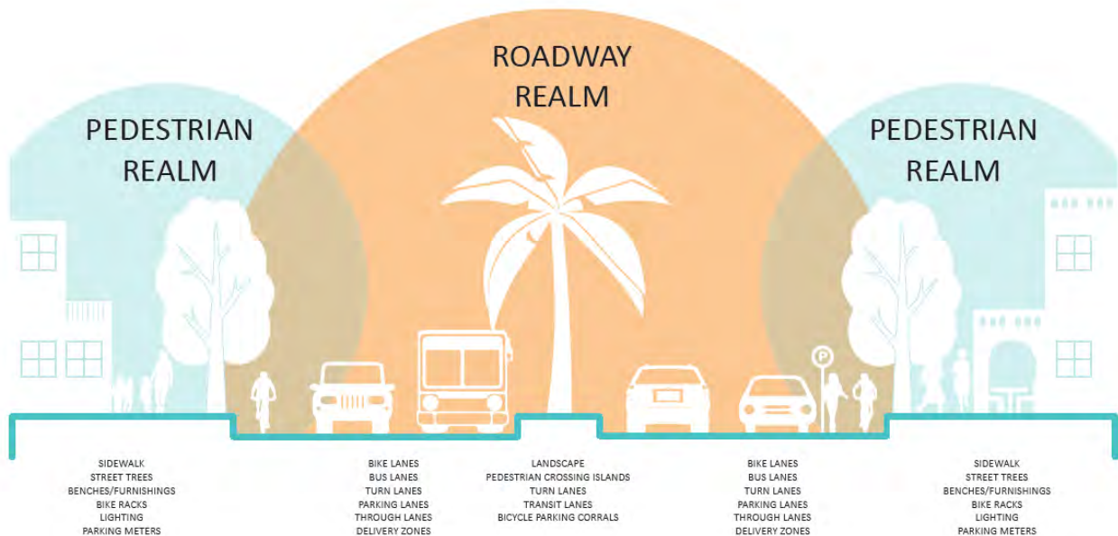
Figure 6: Complete Street Cross Section Elements
